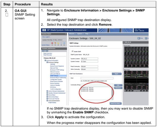
Procedure 51. Delete SNMP Trap Destination on OA
