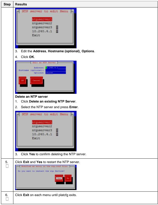
Procedure 96. Configure NTP on TPD-Based Application
