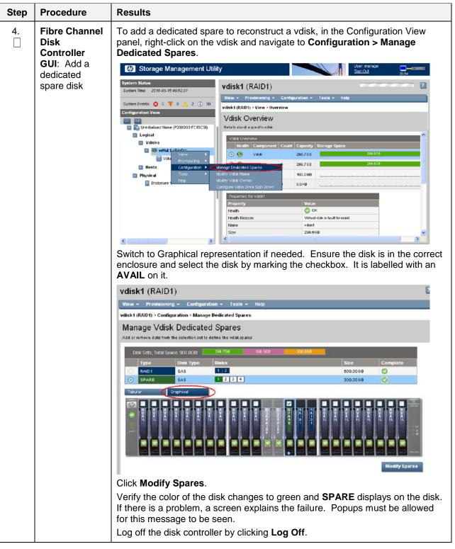
Procedure 33. Replace a Failed Disk in MSA P2000 Disk Array
